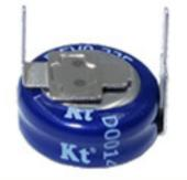
Normal temperature cycle life: 25°C, 500,000 cycles between VR and 1/2VR, Capacity attenuation≤30%, ESR change≤4 times.
